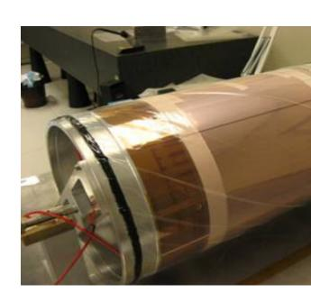
3. The GEM foil is rolled on a mould and then enveloped in
